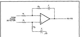
fig. 6. The loop amplifier (integrator) controls the characteristics of the PLL. Loop parameters are set by properly selecting component values. In this balanced configuration, each component appears twice.
